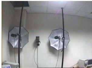
Fig. 1. Diffuse lights and CCD camera
