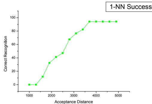
**Fig. 8. Results for 1-NN, train and test with controlled illumination, test images acquired one day later.**
