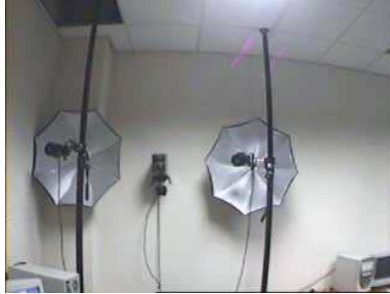
Fig. 1. Experimental set up showing diffuse lighting and the CCD camera.
