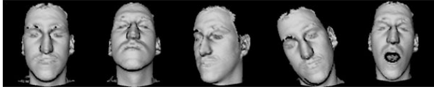
Figure 1 – Sample of 3D meshes from FRAV3D database. From left to right: frontal face, X-axis turn, Y-axis turn, Z-axis turn, face with gesture.
